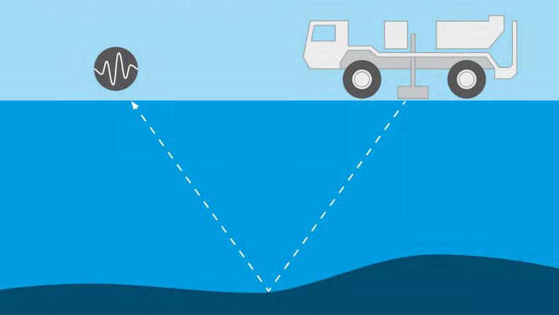
The VibroScan process was developed from 1993 in Austria and is based on the extensive equivalence between train vibrations and sweep experiements.
